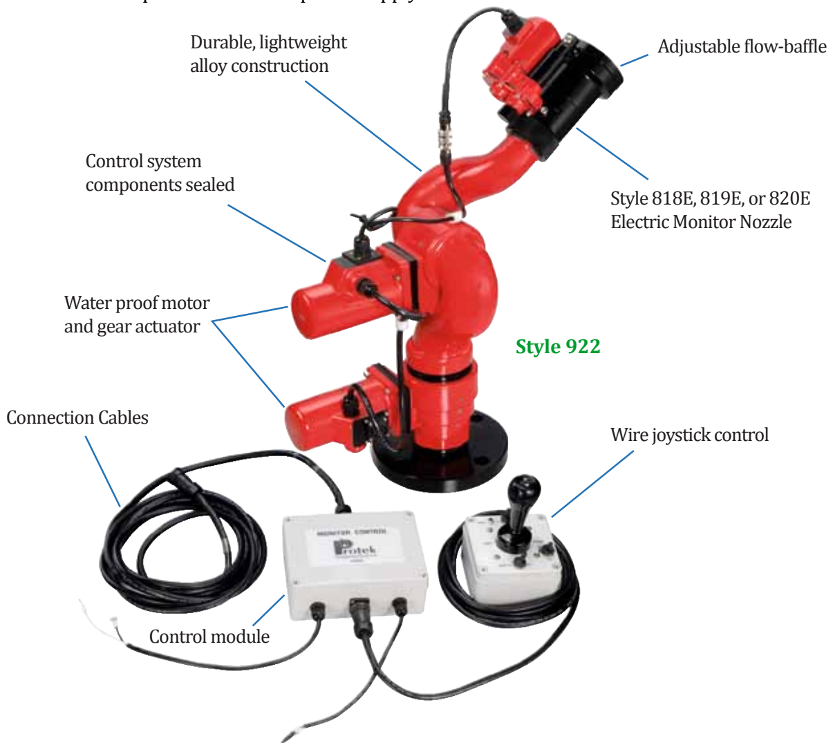
Style 922 monitor shown with standard accessories: Electric nozzle, control module, connection cables, cable joystick control
