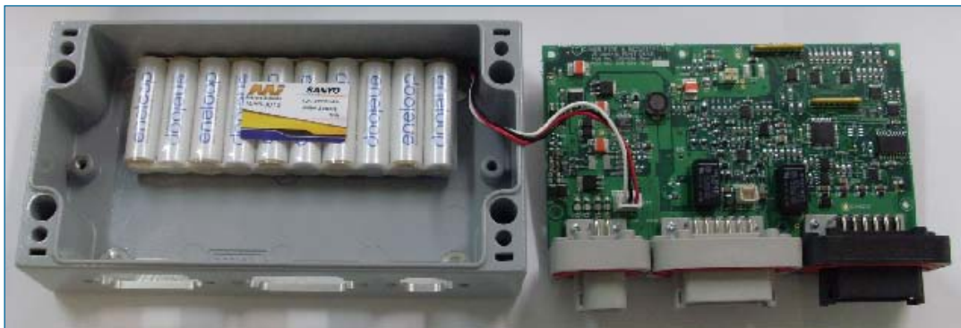
Figure 7 – Back up battery
