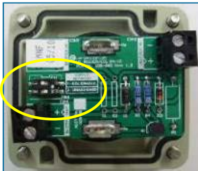
Figure 44 - Audible alarm unit PCB
